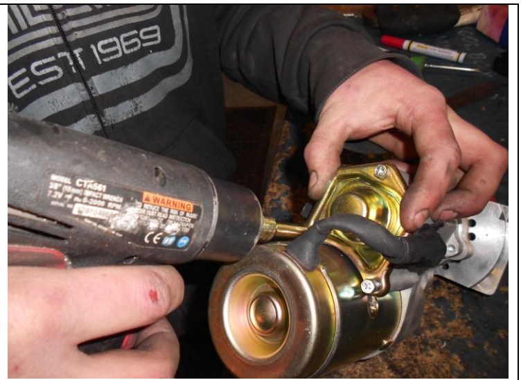
Photo 19 – Refitting the rear plate
