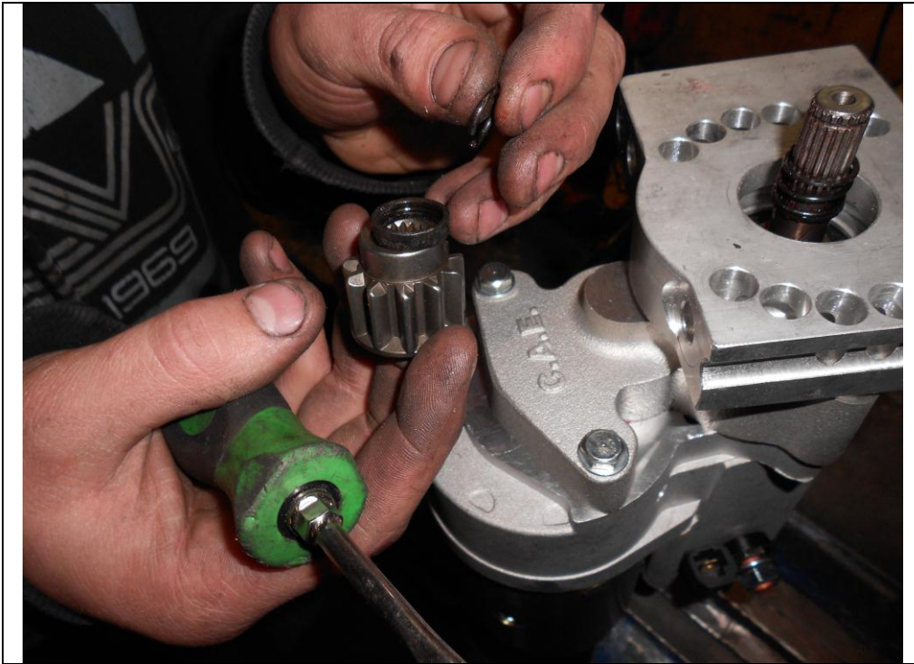
Photo 11 – Removing the pinion, circlip and retainer.
