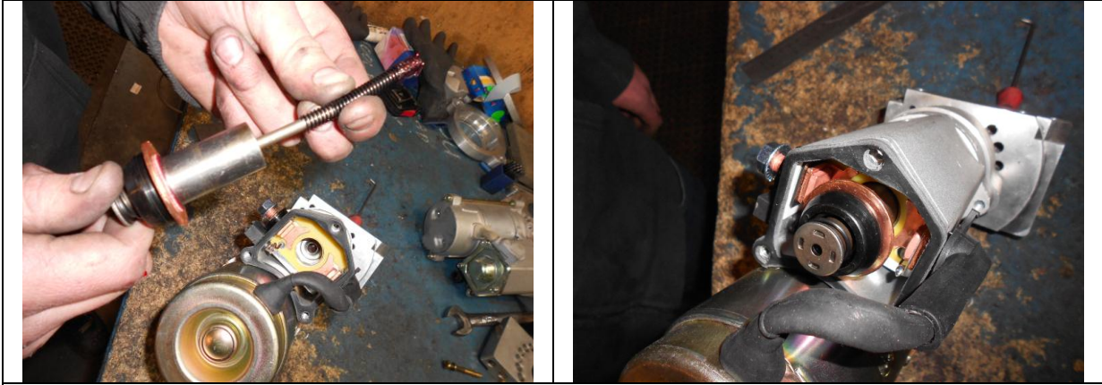
Photo 16 & 17 – Refitting the solenoid plunger and spring
